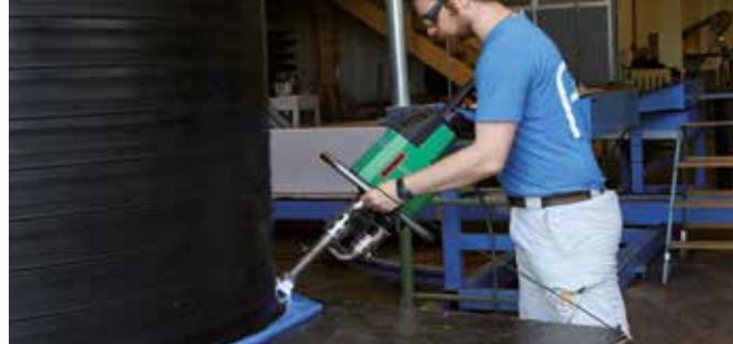
The WELDPLAST S6 is guided easily with the practical control wheel grip.
